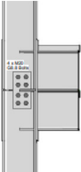
MODULE COLUMN TO MODULE COLUMN CONNECTION SCALE 1:10
