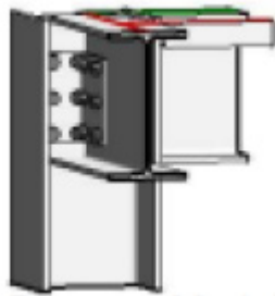
MODULE BEAM TO MODULE COLUMN CONNECTION 1:10
